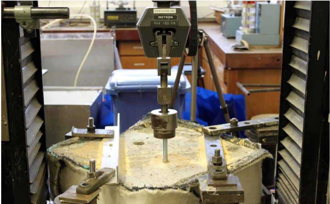
Figure 20: Load testing of fixings for sole-plate into a foam concrete block
